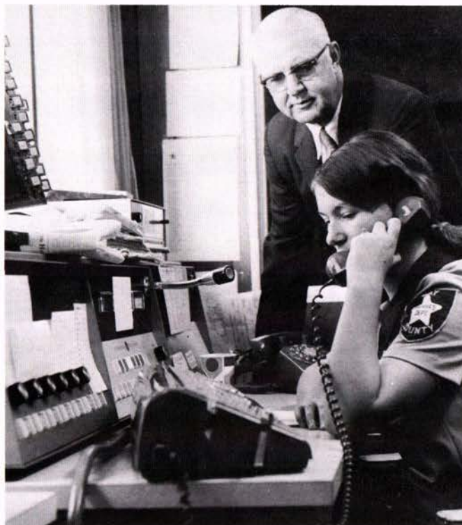
PANAMA CITY — Bay County Sheriff Tullis Easterling is pictured here in his communications control room where two console stations allow two dispatchers to operate simultaneously; and an automatic tape recording device (at the Sheriff's left) records all messages so that the dispatcher is freed from the old system of typing all radio transmissions in a log. The radio dispatcher in the picture is Mrs. Dale Robinson.
