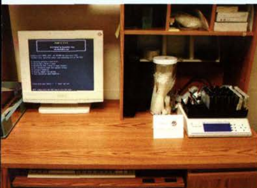
Cleaning workstation, where hard drives are forensically cleaned of all possible data remnants.
